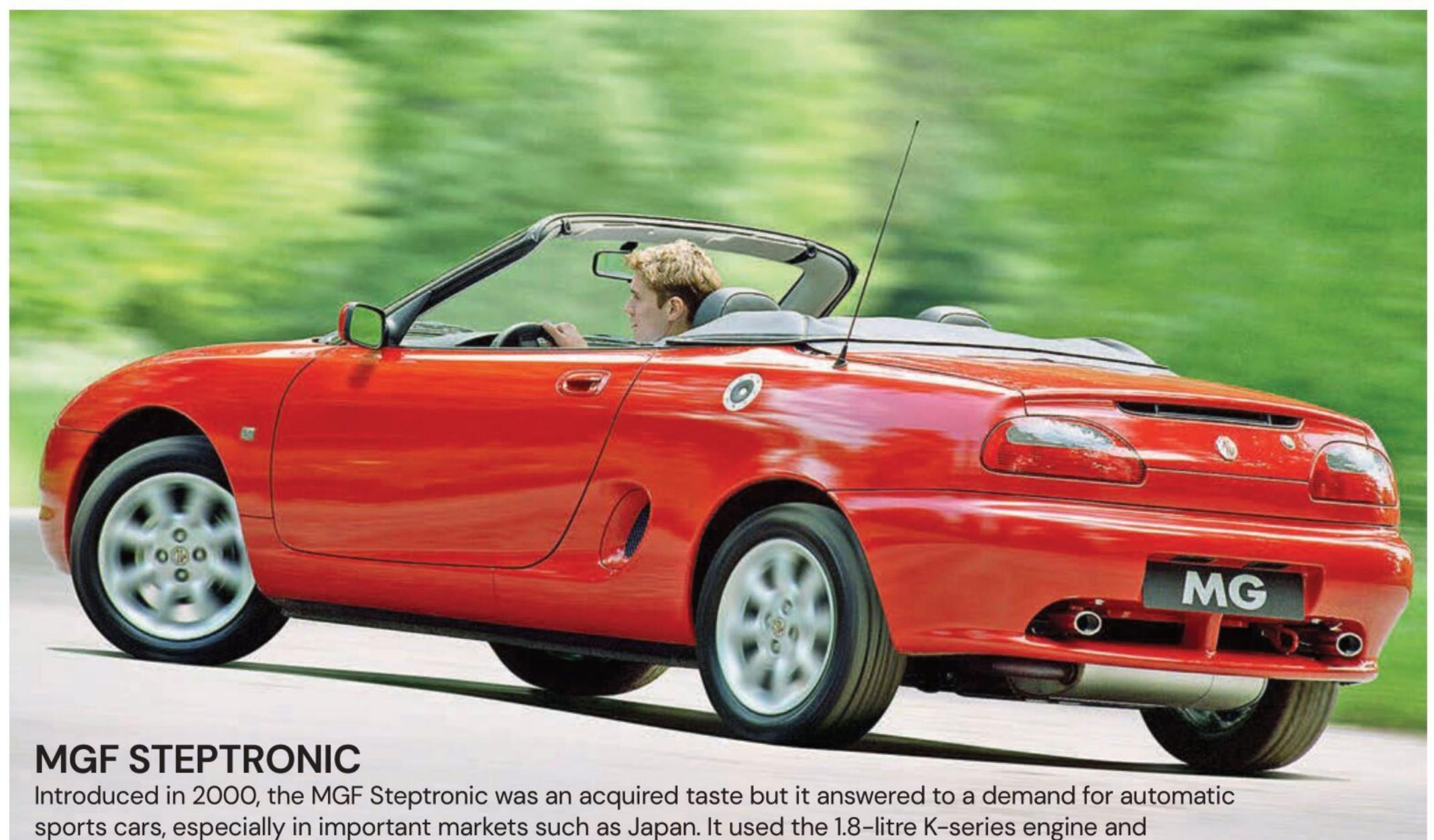
Introduced in 2000, the MGF Steptronic was an acquired taste but it answered to a demand for automatic sports cars, especially in important markets such as Japan. It used the 1.8-litre K-series engine and CVT gearbox combo from the Rover 45, along with steering wheel-mounted buttons to change 'ratios', or at least alter the power delivery from the naturally step-less CVT gear change system.
