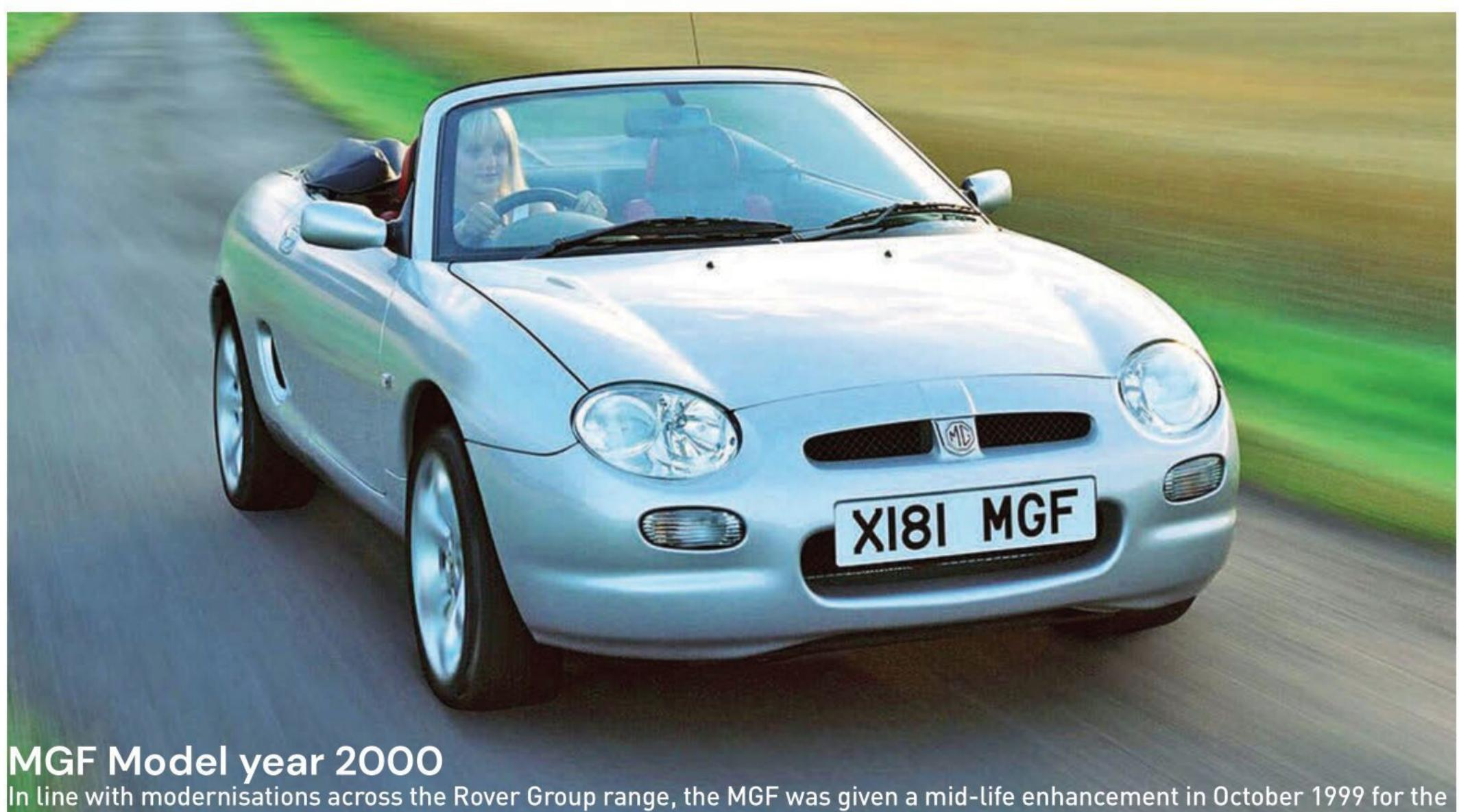
2000 model year. Mechanically there were no changes and visually it was little different, save for clear indicator lenses instead of the original F's orange ones, and a larger rear bumper with aerodynamic diffuser. Inside, the original dials were replaced with more modern ivory clocks, while the mechanical odometer was replaced with a digital one.
