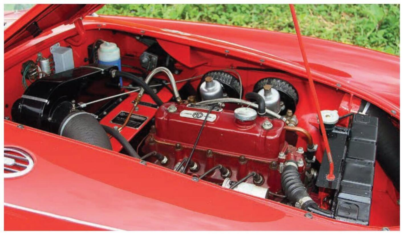
OHV MGA engines were offered in three capacities: 1498cc, 1588cc &1622cc.
