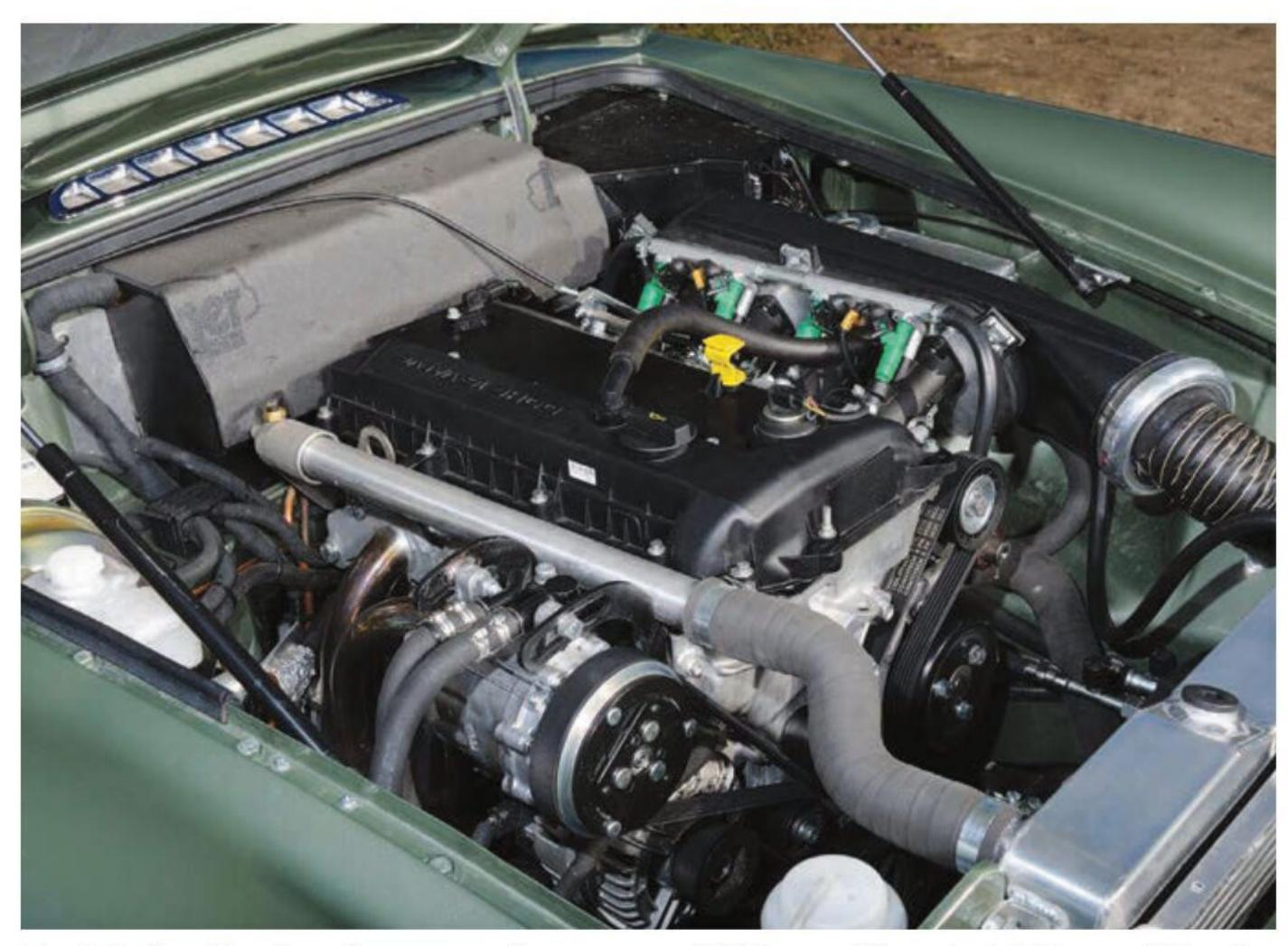
The 2.0-litre Mazda twin-cam engine puts out 214bhp and fires the LE50 up to 60mph in 5 seconds, topping out at 160mph!
