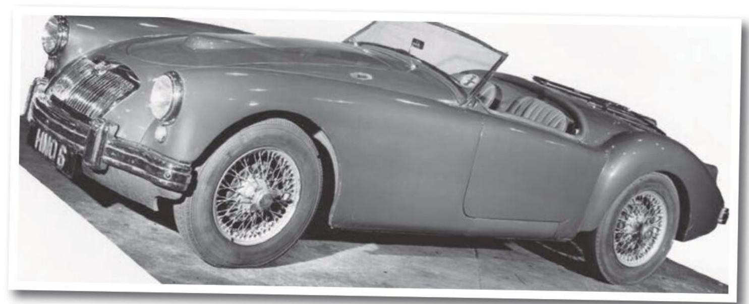
Nearly there. This was the famous EX175 prototype of 1952, looking exactly as the production MGA 1500 became, but fitted with an XPAG TD engine.
