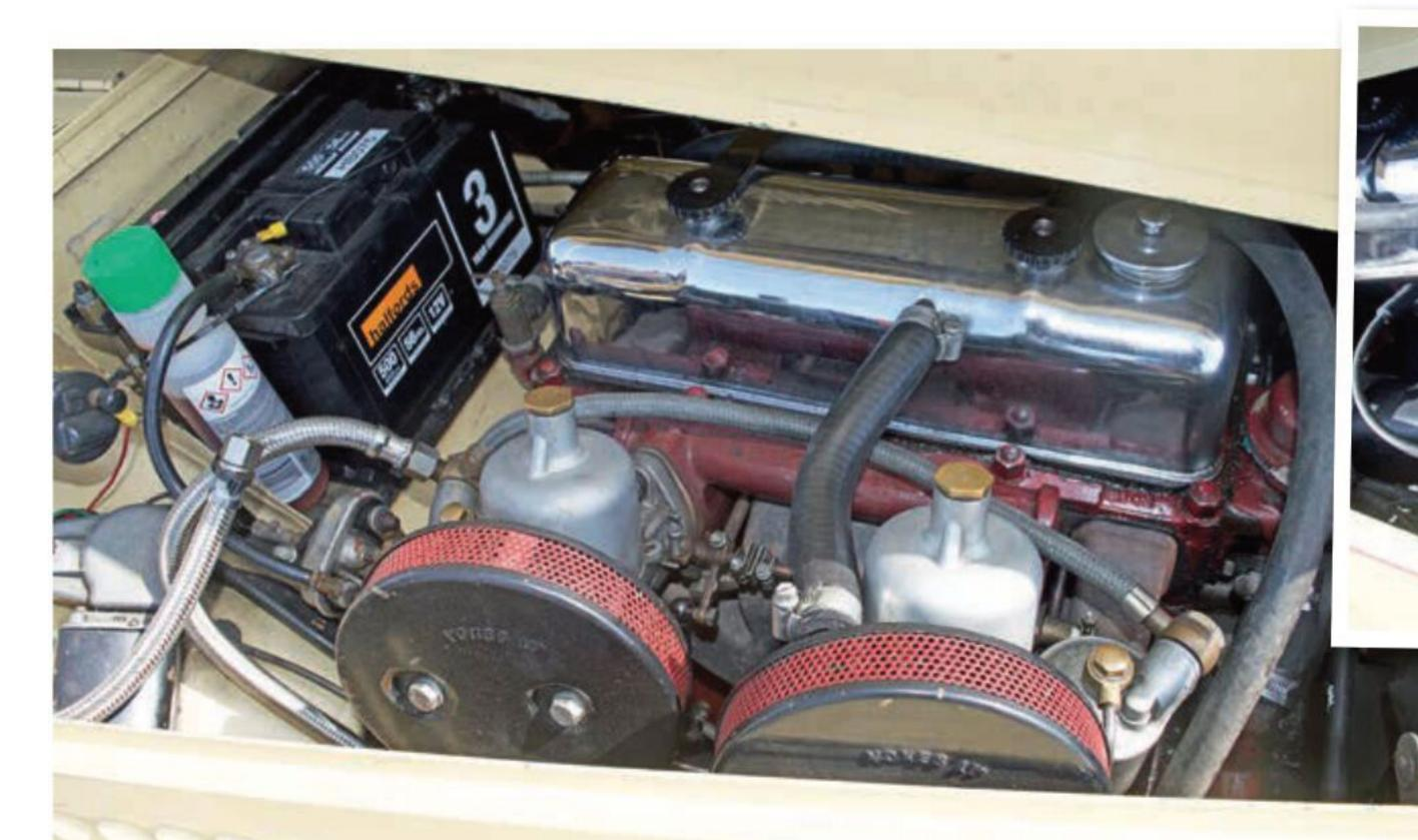
The TF is powered by a 1250cc XPAG engine, fuelled by twin SU carbs.
