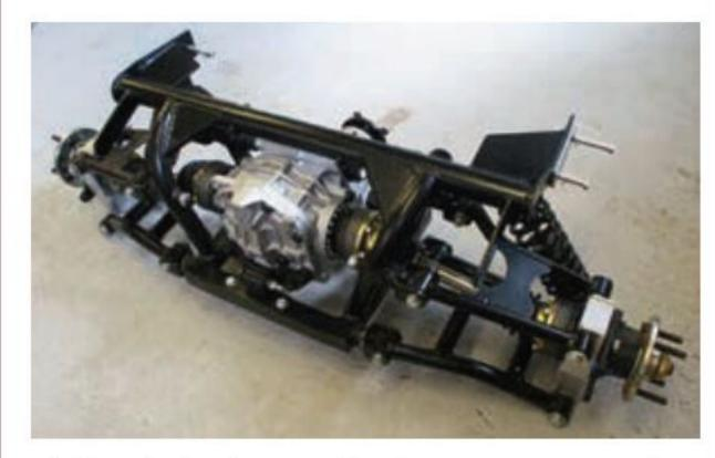
A Hoyle independent rear suspension is highly regarded and will transform the handling of an A.
